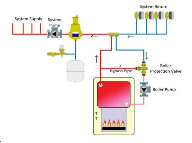
keeping the boiler return at 130 F. As this happens, some hot boiler supply water begins entering the supply tee, where it is mixed with the system water. This slowly adds heat to the system water and brings the temperature of all the radiators up evenly and consistently.
